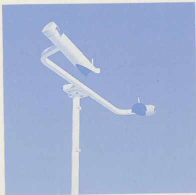
Light-emitting diode weather indicators like this one are a part of the National Weather Service Automated Surface Observing System (ASOS) weather stations.
