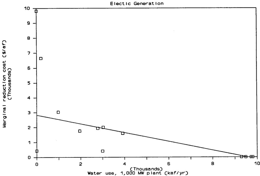
**Figure 4.2.** Estimation of demand for cooling water.
