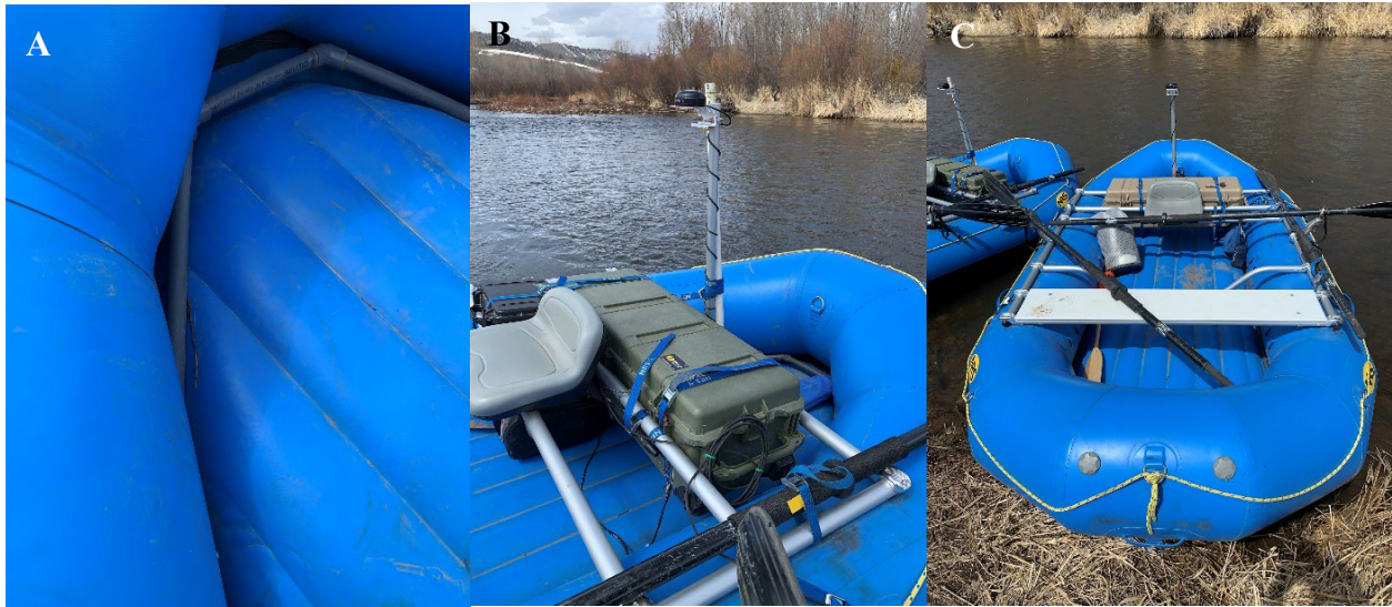
Figure 2.16. (A) Antenna wire encased in PVC to maintain rigidity, shape, and tuning during deployment. (B) Pelican box, containing batteries, reader, tuner box, and Campbell Scientific datalogger, and external GPS unit for marking the location of detected PIT tags. (C) Portable antennas set to deploy on the Fraser River Ranch.
