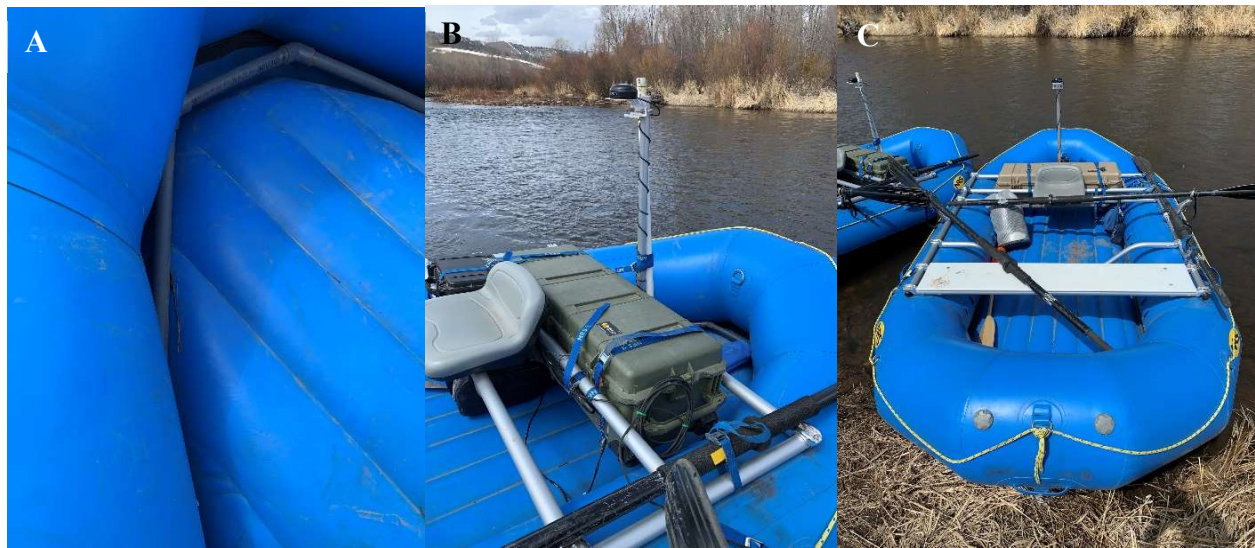
Figure 2.17. (A) Antenna wire encased in PVC to maintain rigidity, shape, and tuning during deployment. (B) Pelican box, containing batteries, reader, tuner box, and Campbell Scientific datalogger, and external GPS unit for marking the location of detected PIT tags. (C) Portable antennas set to deploy on the Fraser River Ranch.
