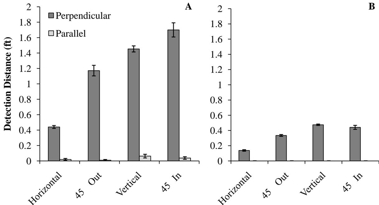
**Figure 2.13.** Average maximum detection distances ( $\pm$  SE) for the 6 AWG, 100-foot antenna with 32 mm (panel A) and 12 mm (panel B) PIT tags oriented perpendicular and parallel to the antenna wire in the horizontal, 45° outward, vertical, and 45° inward detection planes.
