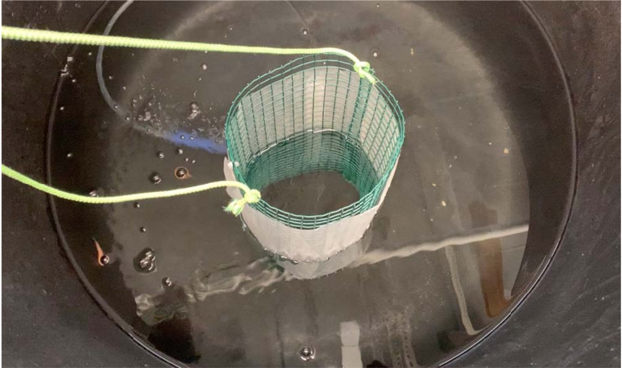
Figure A2: The 204 L predator cage with wire/mesh 175 mm diameter inner cage. Attached cord allows trial to be started by technician from behind curtains.
