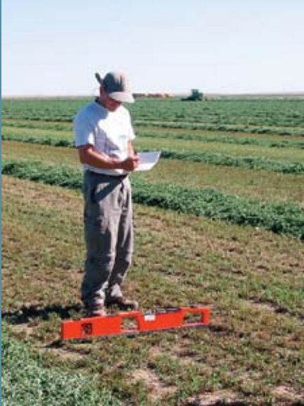
Geonics™ EM-38 electromagnetic induction meters (Rhoades et al. 1999) were used to gather soil salinity data within selected fields.
