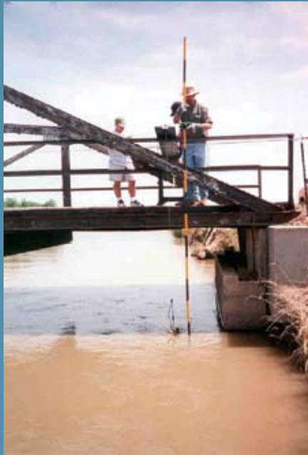
Inflow-outflow tests for seepage have been conducted in the Rocky Ford Highline Canal, the Catlin Canal, and the Fort Lyon Canal in the Upstream Study Region.
