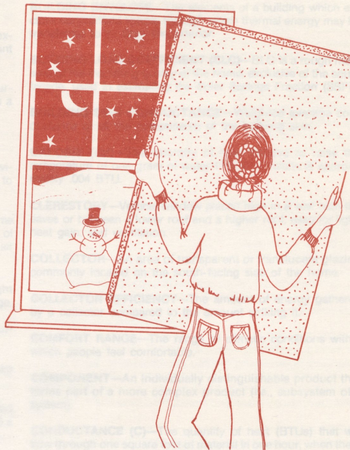
Movable Insulation Night Wall
