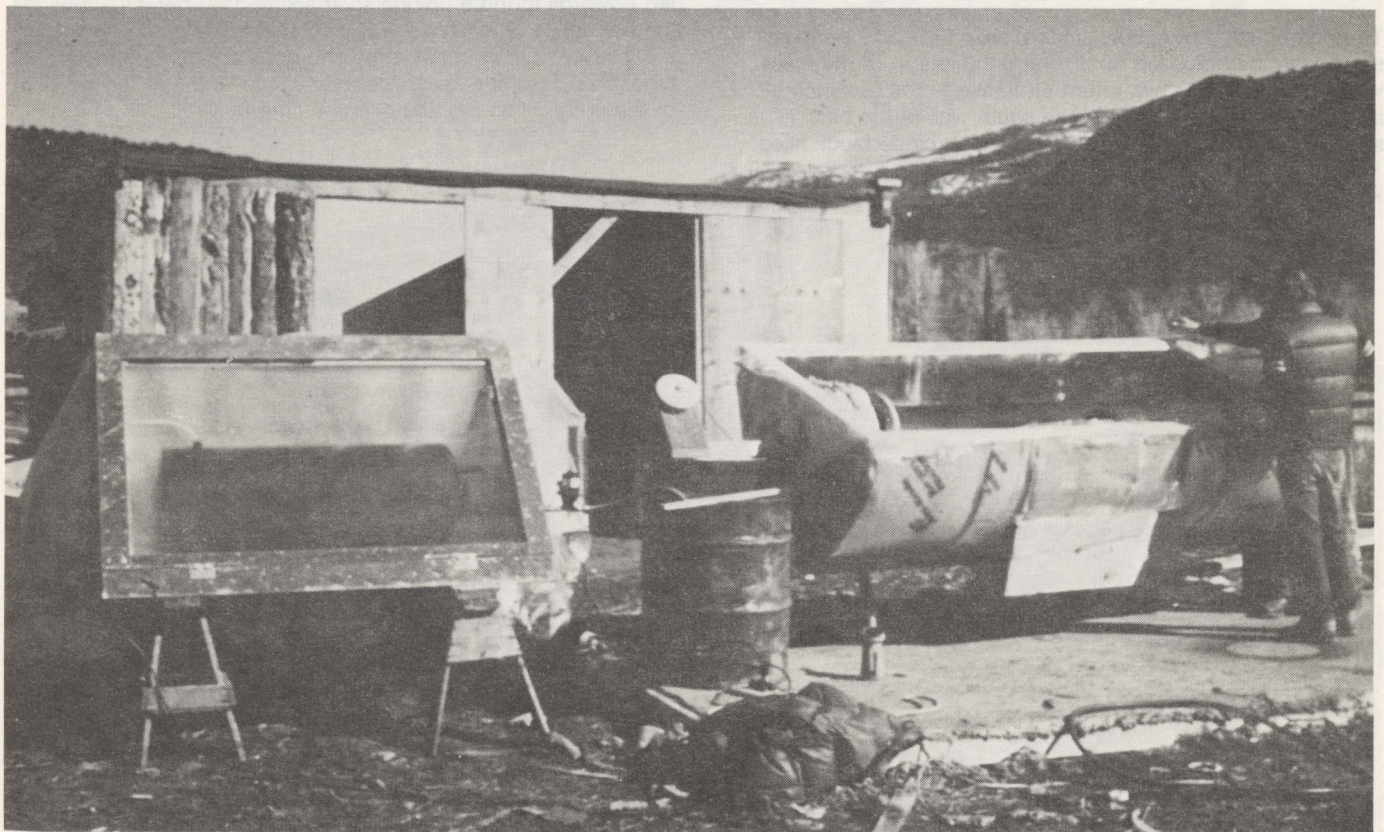
"Two different types of "breadbox" water heaters are compared. The parabolic heater, on the right, appears to be out-performing the conventional breadbox heater on the left."
