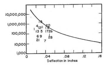
Study are superimposed on the graph as site numbers. Most roadways investigated for this Colorado study were structurally weaker than the AASHO Road Test designs and only 1/3 of them were down to the 2.5 PSI level, so most of the points on the graph fall below the AASHO line.
