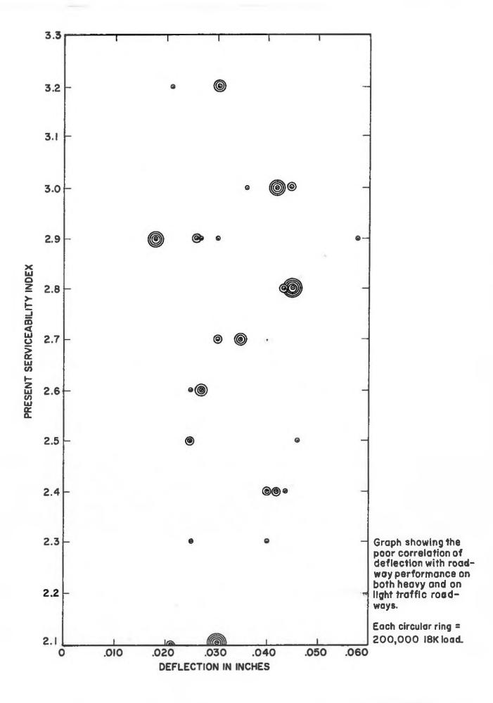
AASHO Road Test findings are shown on the adjoining figure. The number of 18K repetitions to reduce a flexible pavement to the 2.5 PSI condition is shown at the left for a corresponding deflection.
