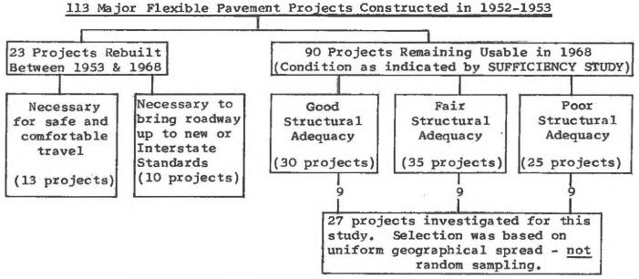
The 27 projects studied were probably as representative of the 90 surviving projects as can be found. On the other hand, these projects reveal very little about the cause of the failures of the 13 projects which had to be rebuilt for safe and comfortable travel. These 13 rebuilt projects may be placed in the following categories:
