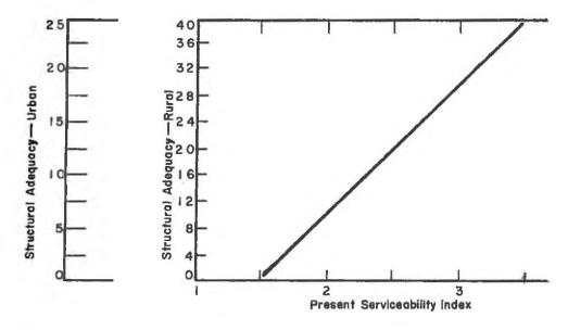
This bit of information may be quite valuable in that it can be used to statistically determine structural adequacy for the Colorado Sufficiency Report when the Present Serviceability Index Value is known. Recent developments indicate that the PSI can be determined with the CHLOE or the Colorado Accelerometer and thereby make it possible to get Structural Adequacy by a mechanical means rather than by human judgment in 1971 when the next evaluation is made.
