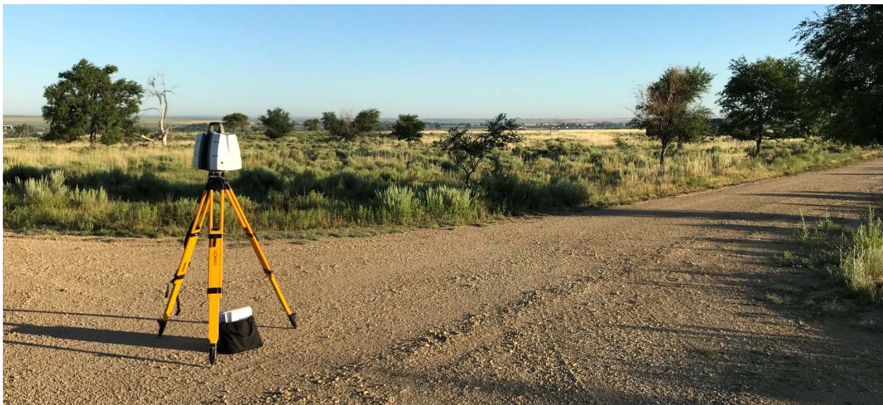
Leica Scan Station P50 located at intersection of the Amache Japanese American Confinement Site.
