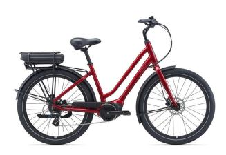
The Momentum LaFree E+ (pictured) is a Class 1 eBike. A battery above the wheel and electric motor attached to the pedals provides assistance up to 20 miles per hour (mph) and only when a rider is pedaling. The bike has five different levels of assist and can travel up to 65 miles on a single charge.
