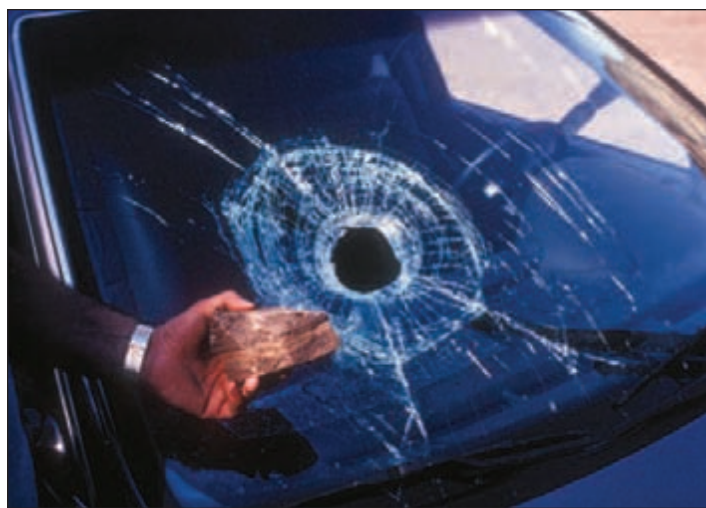
Figure 1: Rockfall accident in Glenwood Canyon. This hand-sized rock free fell 300 feet before striking the vehicle. The driver was unhurt and, luckily, there was no front seat passenger. (Photo by Jon White.)
