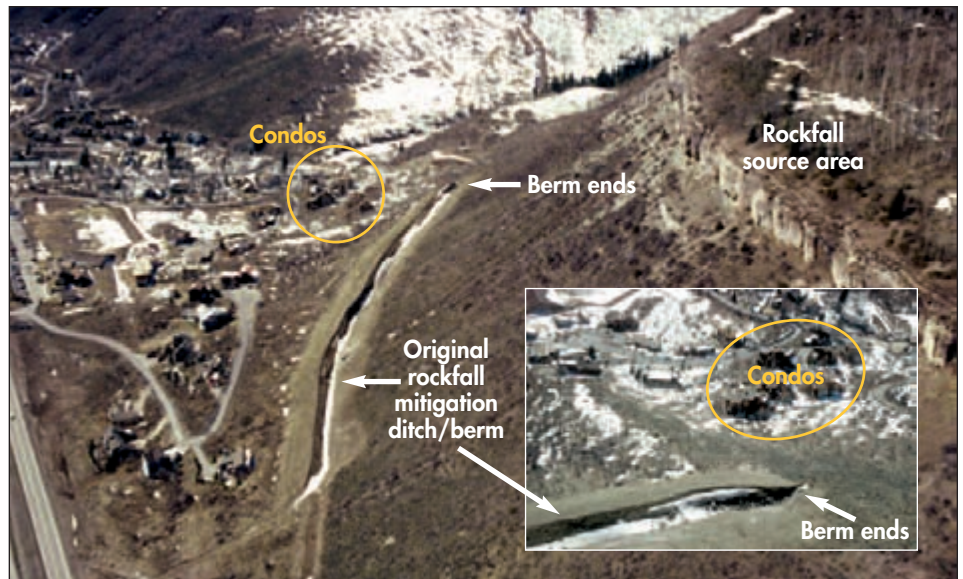
Figure D: Oblique aerial view, looking west, of Booth Creek debouching onto the Vail Valley floor. Interstate 70 highway is shown on the far lower left of the photo. The ditch and berm completed in 1990 is shown left of center. The termination of the berm and continued rockfall-hazard exposure of the condos (circled in yellow) is shown in the inset photo. (Photos by Jon White.)
