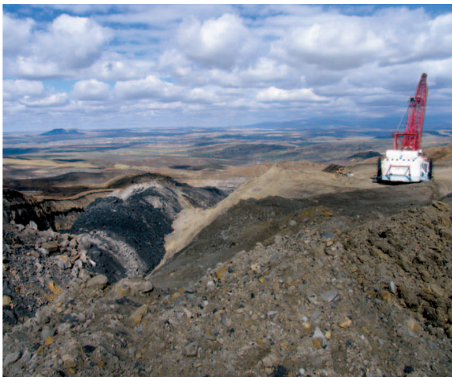
Figure 35. Baby Doe Dragline at the Trapper Mine moving from the G dip line pit, October 2006. Landslide ridge in pit floor seen at left.
