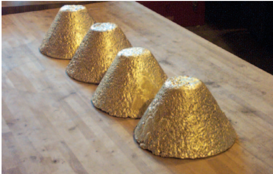
Figure 49. Production at the Cripple Creek & Victor facilities of gold doré buttons produced by CC&V. The buttons weigh 65–70 pounds, and are composed of 65 to 70 percent gold, with the rest silver. The typical weight is around 650 ounces of gold and 200 ounces of silver worth nearly $500,000 each. (Photo courtesy of Cripple Creek and Victor Corp.)
