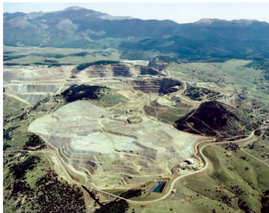
Figure 48. Aerial view of the Cripple Creek & Victor Mining Company operations in Teller County. The heap leach pad and State Highway 67 are in the foreground, the open-pit mines are behind and above the pads. The town of Victor is to the right of the mine and Pikes Peak is in the background. (Photo courtesy of AngloAshanti Gold Corp.)
