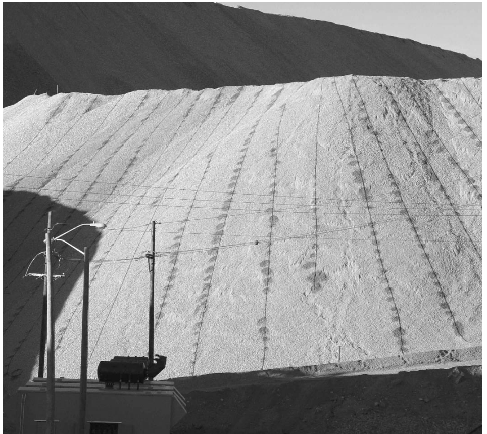
Heap leach pad with a drip system that gently applies a solution of water and sodium cyanide to crushed and screened gold ore at the Cripple Creek & Victor Gold Mine.
