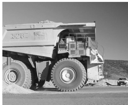
Massive new truck at the Cripple Creek & Victor with the capacity to haul 310 tons of ore per load.
