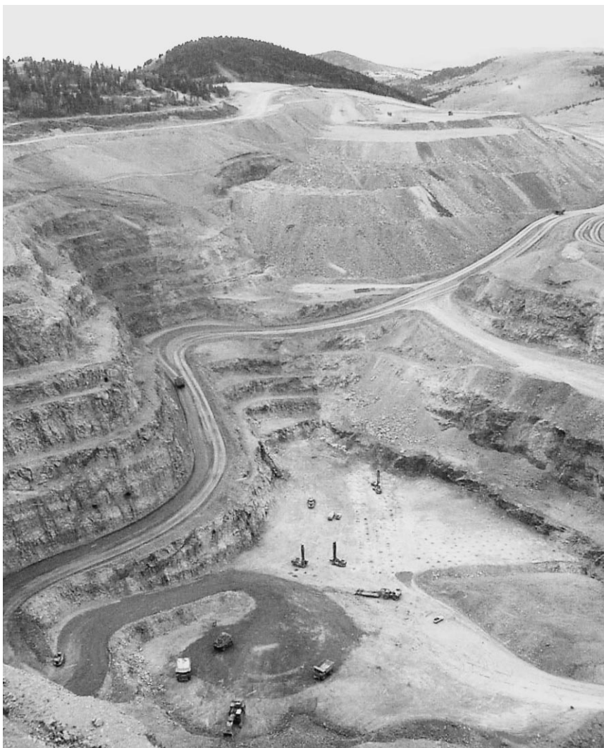
The Cripple Creek & Victor gold mine. Note the drilling rigs forming a blasthole pattern in the bottom of the mine.
