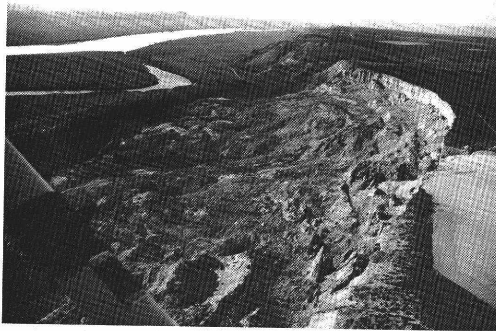
Figure 6. Aerial view of the Savage Island landslide on the east shore of the Columbia River, Washington, 1981. This landslide was caused by irrigation water (photograph by Robert L. Schuster, U.S. Geological Survey).
