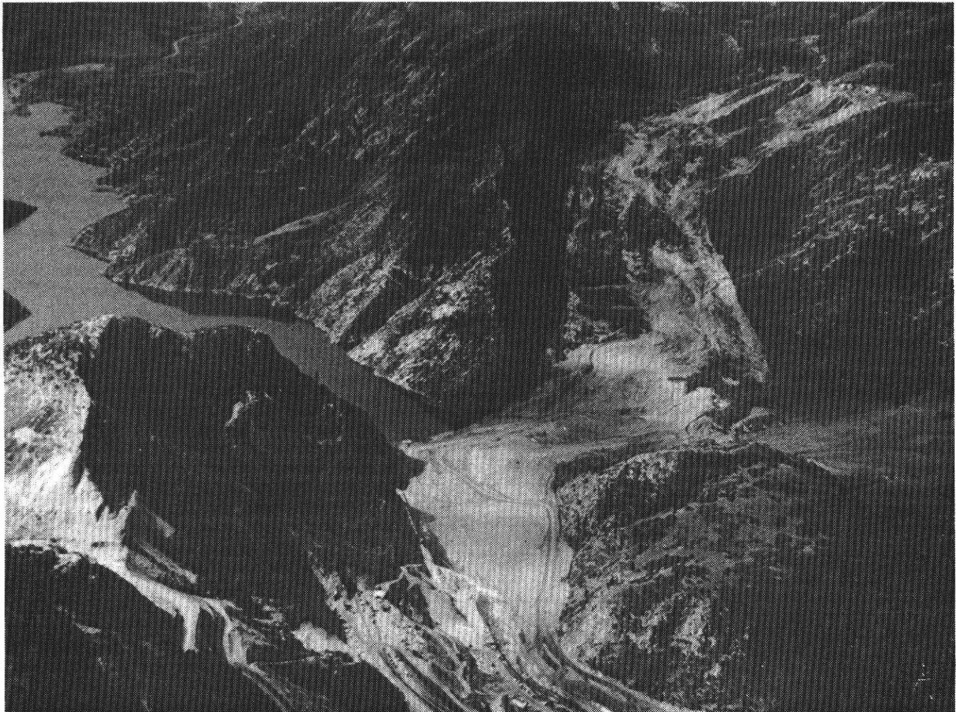
Figure 19. Aerial view of the Thistle landslide, Utah, 1983. This landslide dammed the Spanish Fork River creating a lake which inundated the town of Thistle and severed three major transportation arteries (photograph by Robert L. Schuster, U.S. Geological Survey).
