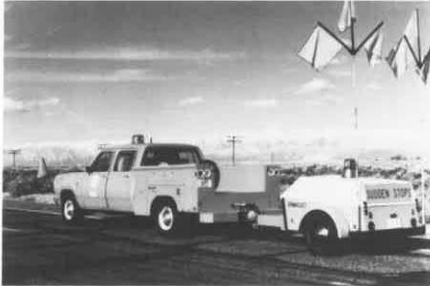
Photograph 1 - Dynaflect Trailer and Tow Vehicle
