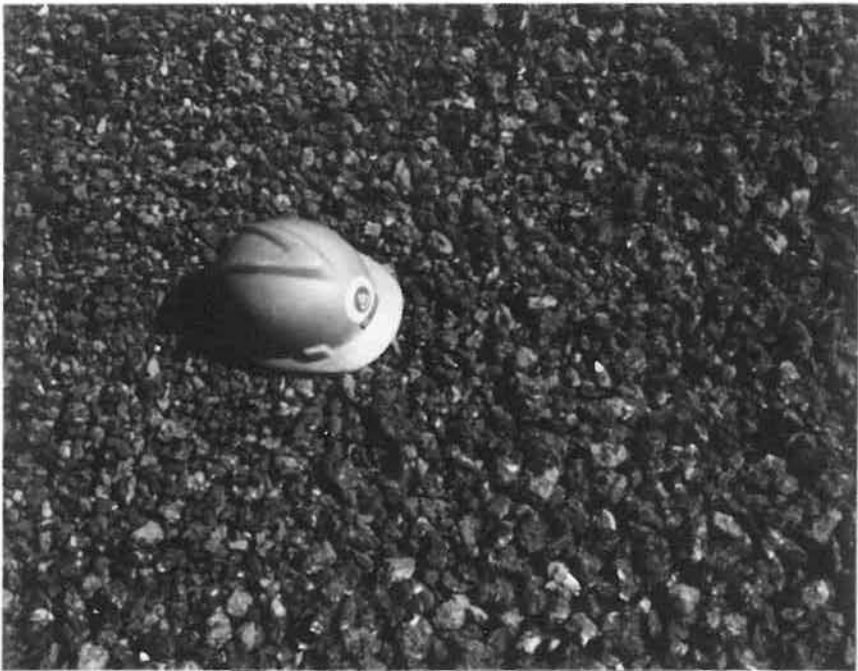
Photograph No. 6 Crushed pavement stockpile. Note: minimal contamination.
