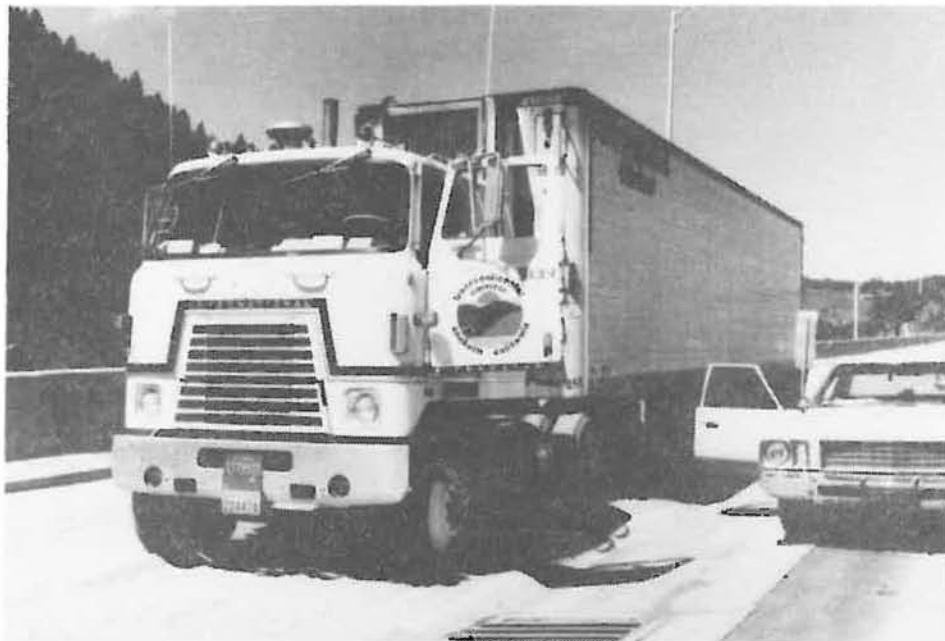
Truck safely stopped after travelling 800 feet through the gravel.
