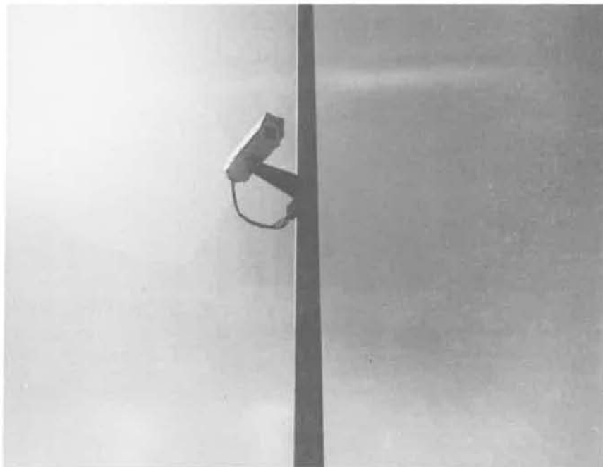
One of four video cameras that were used to record trucks using the escape ramp.
