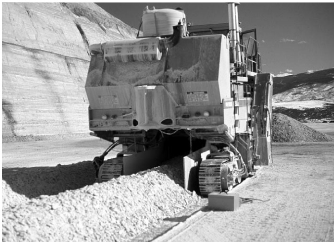
Pavement-profiler machine mining gypsum at the American Gypsum Mine in Eagle County, Colorado. The gypsum is used to make drywall at a plant in the nearby town of Gypsum.
