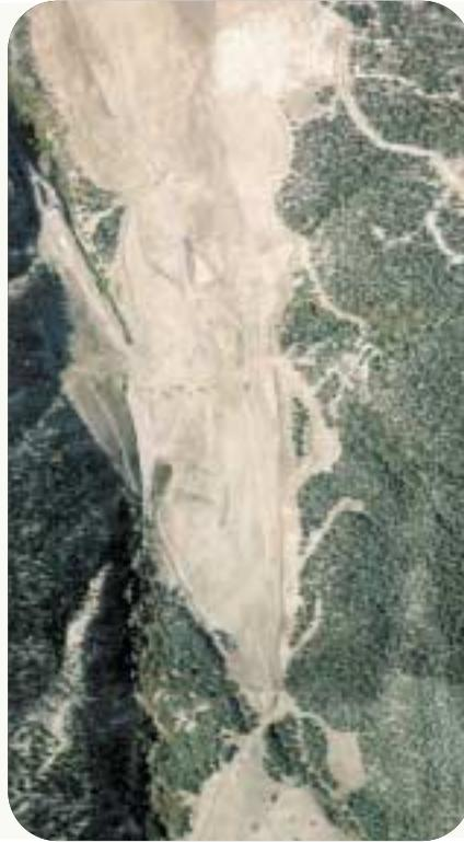
*Phase I bond release was granted following backfilling and grading of the mine site and drainage reestablishment. Topsoiling and revegetation are in process.*
