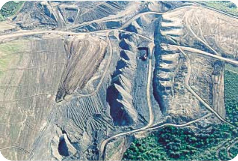
*Left: Inspections include sampling for vegetative cover. Above: This photo shows the stages of mining and reclamation in a surface coal mine. From left to right: revegetation after two growing seasons; revegetation after one growing season; replaced topsoil; regraded spoil; spoil ridge; open pit; disturbed lands where topsoil has been salvaged. Right: Sampling mine discharge is often part of the monthly inspection routine.*
