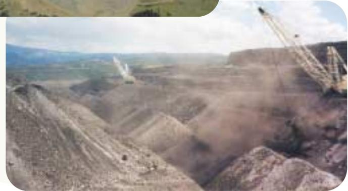
*From Top: Coal crushing facility in Gunnison County; Cripple Creek and Victor Gold Mining Company near Victor; Overburden spoil ridges at a surface coal mine in Northwest Colorado.*
