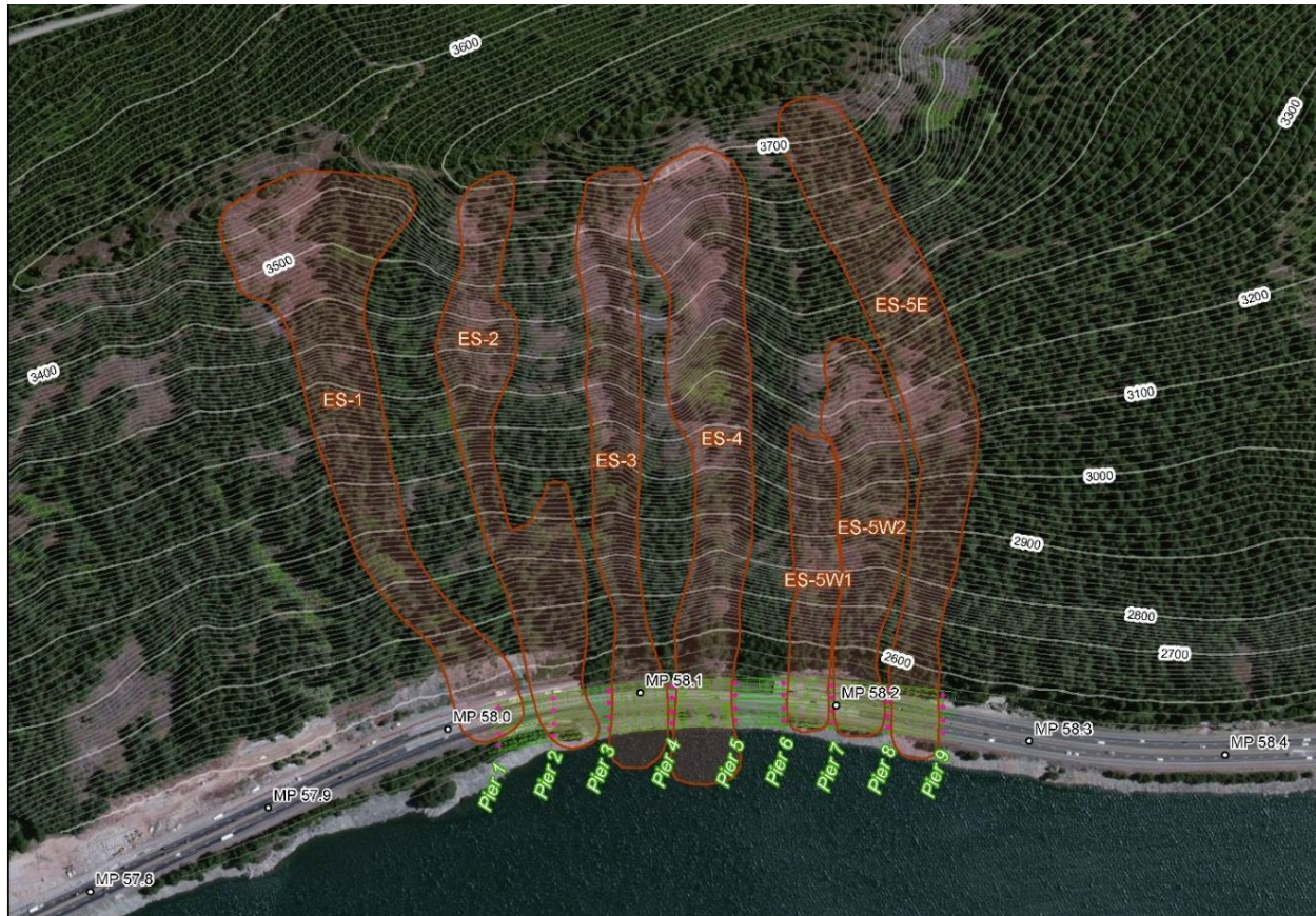
Figure 44: East Shed project area overview showing location of current highway, Keechelus Lake, seven East Shed avalanche paths, and proposed locations of bridges (green lines) and piers (pink dots) (from Jones et al., 2014)
