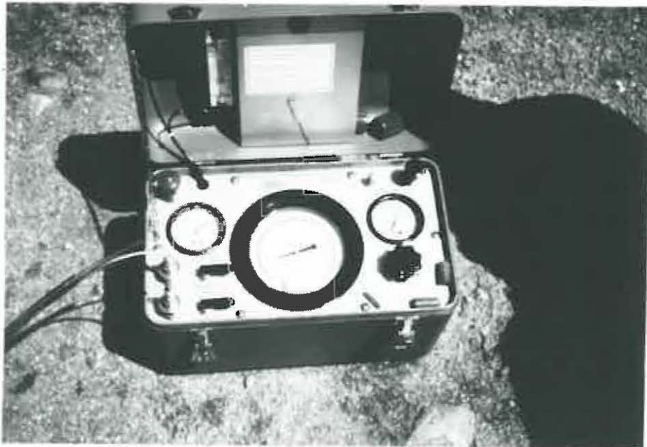
FIGURE 17. READ-OUT DEVICE FOR THE PNEUMATIC PIEZOMETER
