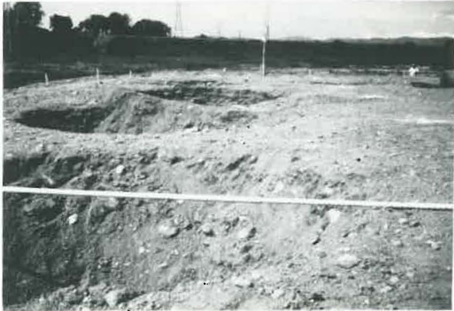
FIGURE 27. DIAMETERS OF CRATERS WERE MEASURED TO BE 10 TO 12 FEET AT THE END OF THE PRIMARY PHASE
