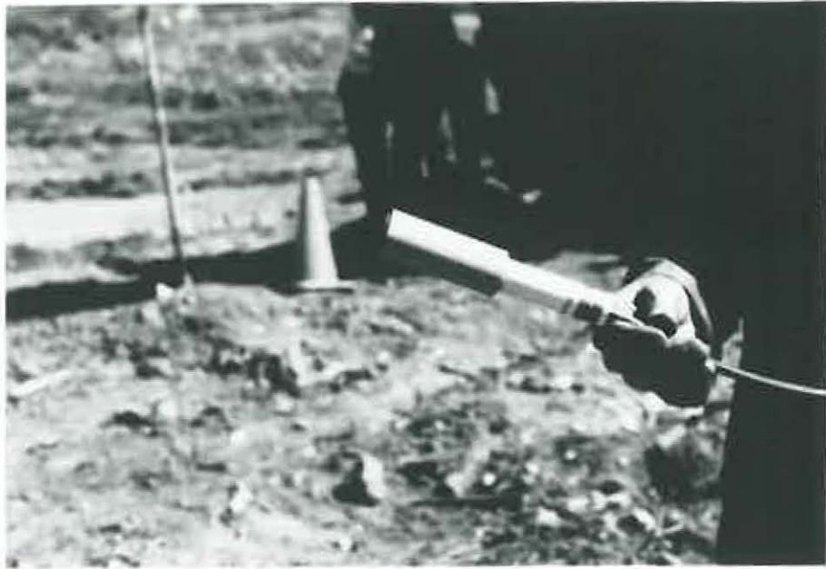
FIGURE 16. PNEUMATIC PIEZOMETER MANUFACTURED BY THE SINCO COMPANY
