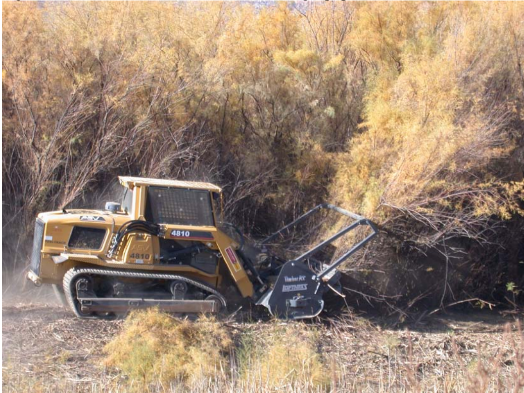
Figure 10: Medium-sized mechanized mulching equipment
