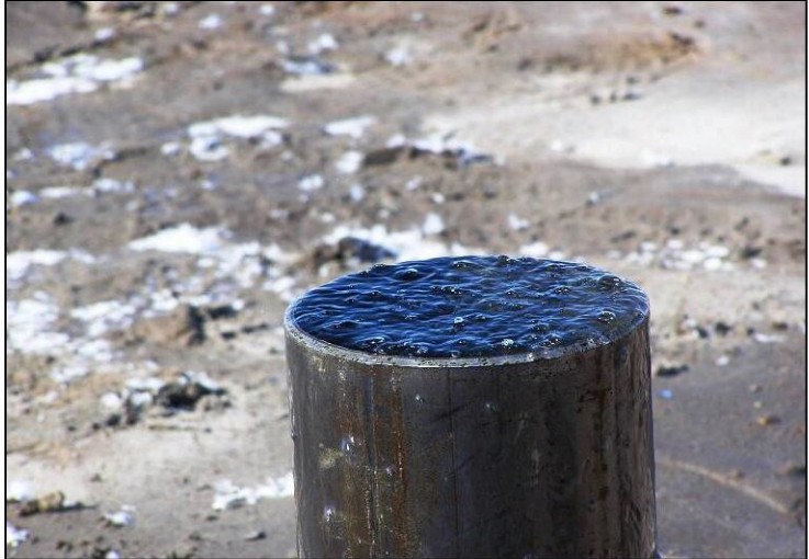
Gas bubbling from a new well. (Photo by Larry Hakes, Well Inspector)
