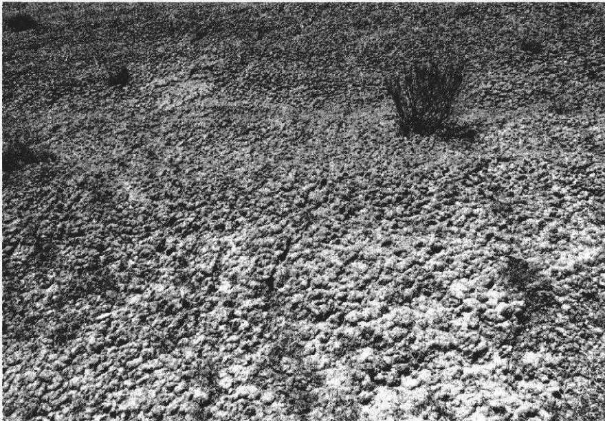
When they are dry, swelling soils often can be recognized by their "popcorn" appearance.
