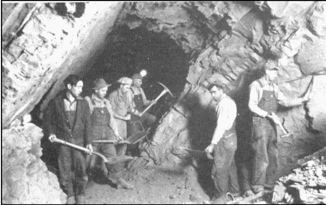
Miners at work in an underground pottery clay mine in Jefferson County (1940s). Note the steep dip to the left (east) of the sedimentary beds.
