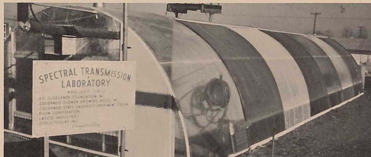
Transmission characteristics of fiberglass reinforced plastic sample are being determined with a recording spectroradiometer.
