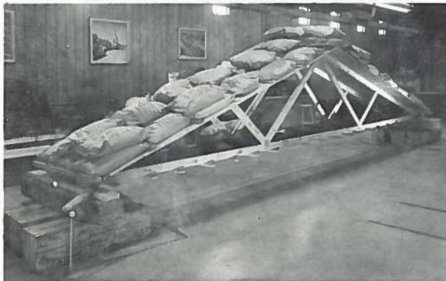
Test stands such as this one were made to show Colorado woods exceeded minimum construction specification. Test results have gained increased acceptance and use of Colorado forest products.
