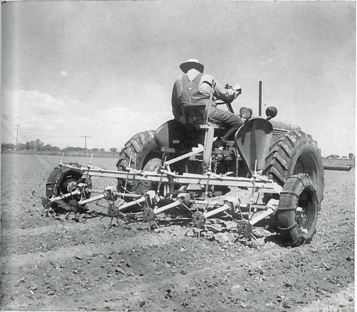
Sugar beet thinners like the one shown here are helping Colorado sugar beet growers cut down labor costs. Mechanical thinners were used on nearly 60 percent of the state's sugar beet crop last year.
