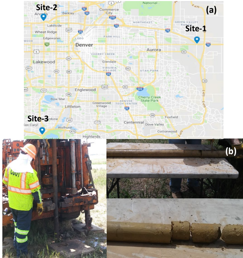
Figure 1. Sample drilling sites: (a) location on the map; (b) drilling pictures from site-1.
