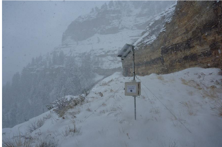
Acoustic detector deployed in front of Gate 3 at Anvil Points Mine during the winter of 2017.
