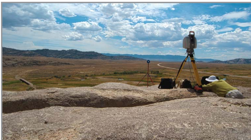
Mike Nulty operating scanner at the top of Independence Rock
