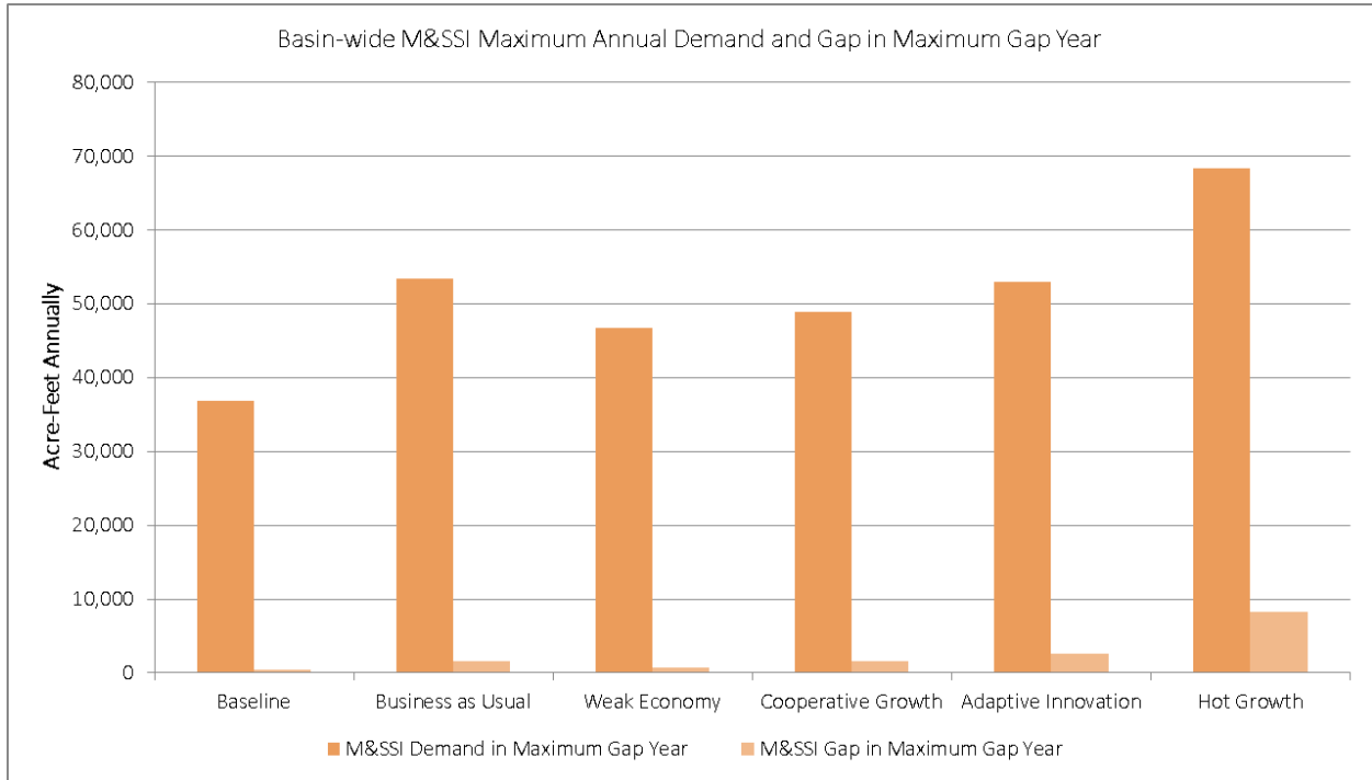
Figure 147: Yampa River Basin M&SSI Maximum Annual Demand and Gap in Maximum Gap Year
