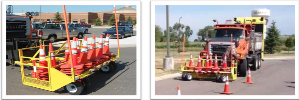
Figure 21. MnDOT TTCD cart (47).
