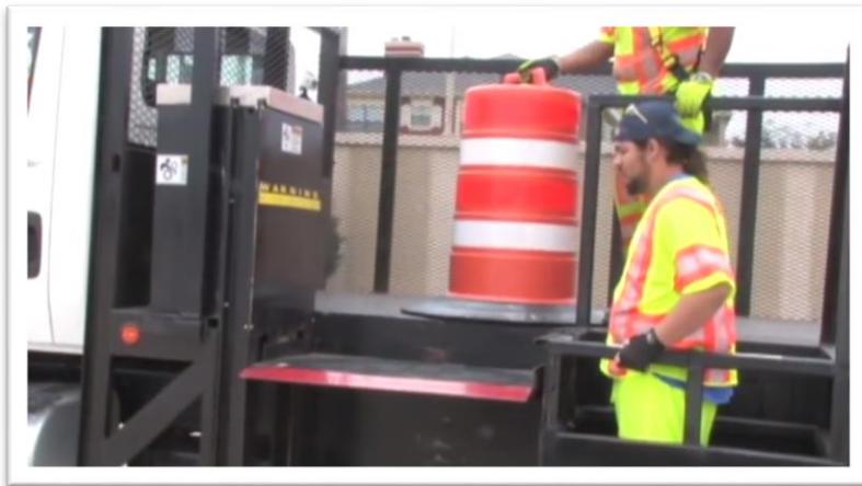
Figure 27. NTTA Hydraulic deck for lowering and lifting devices (51).
