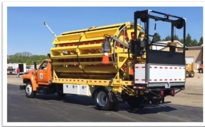
Figure 5. MnDOT AutoCone 500 truck (16).
