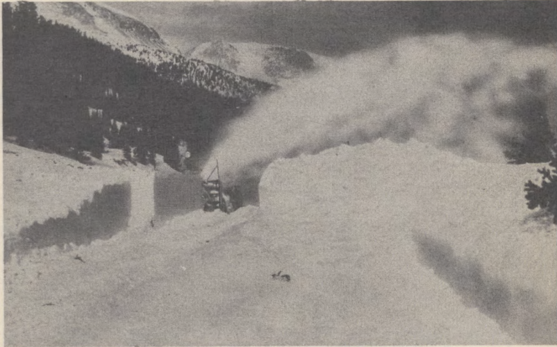
Rotary plows buck the big drifts, clearing highways for cars and trucks.
