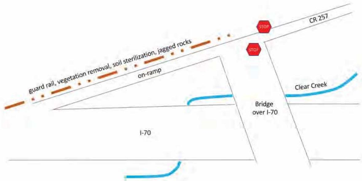
*Figure:* Conceptual drawing of mitigation components at MP 231.2, the Empire on-ramp onto westbound I-70.
