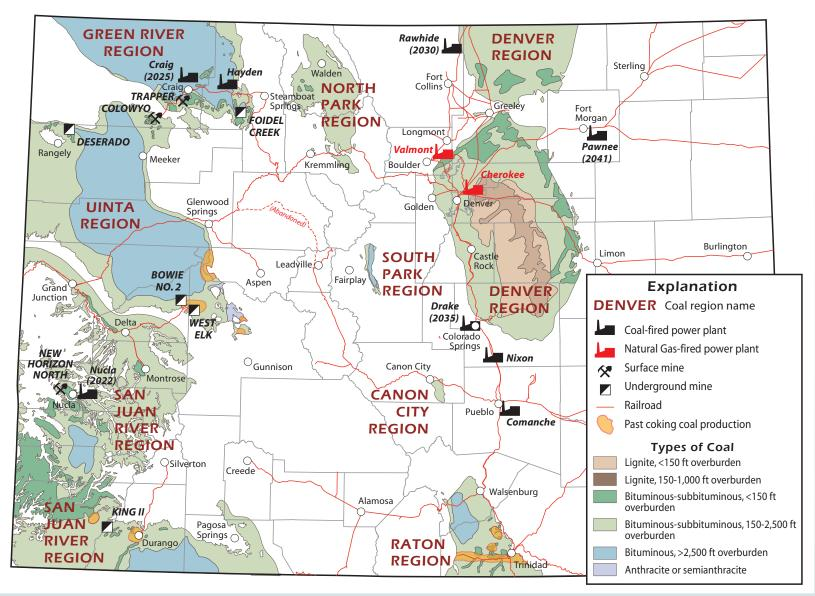
Figure 2-5. Locations of active coal mines, power plants, railroads, and coal-bearing regions in Colorado, 2016. Dates in parenthesis are estimated closure dates for given power plants.
