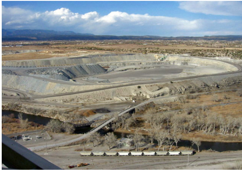
High view of Holcim (US) Inc's limestone and shale surface mine, Fremont County. Photo John Keller archive.
