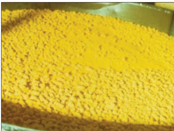
Figure 53. Uranium ore arrives at the mill containing less than 1 percent uranium. Through the milling process, yellowcake is produced—a powder of consisting of approximately 90% U_3O_8 , with about 0.3% of the fissionable isotope U-235. The yellowcake is then shipped to a plant where the concentration of U-235 is raised to about 4% for use in fuel rods for nuclear power plants.
