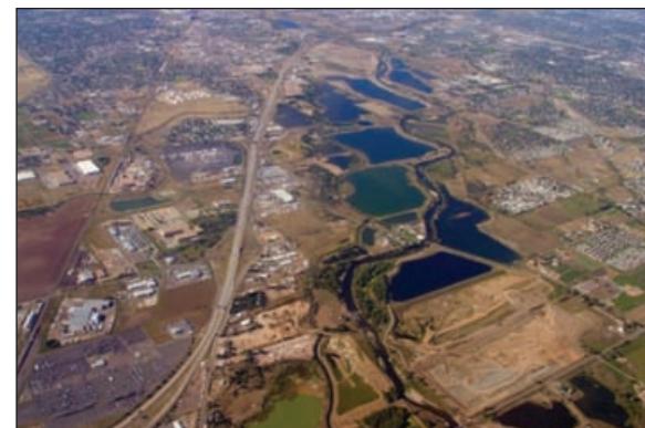
Figure 75. Aerial view of gravel pits along the South Platte River in Adams County. The alluvial (river-laid) sand and gravel deposits along the Front Range have been mined for years to provide aggregate used for construction and development in the metro area. Many of the quarries remain as ponds after mining is completed.
