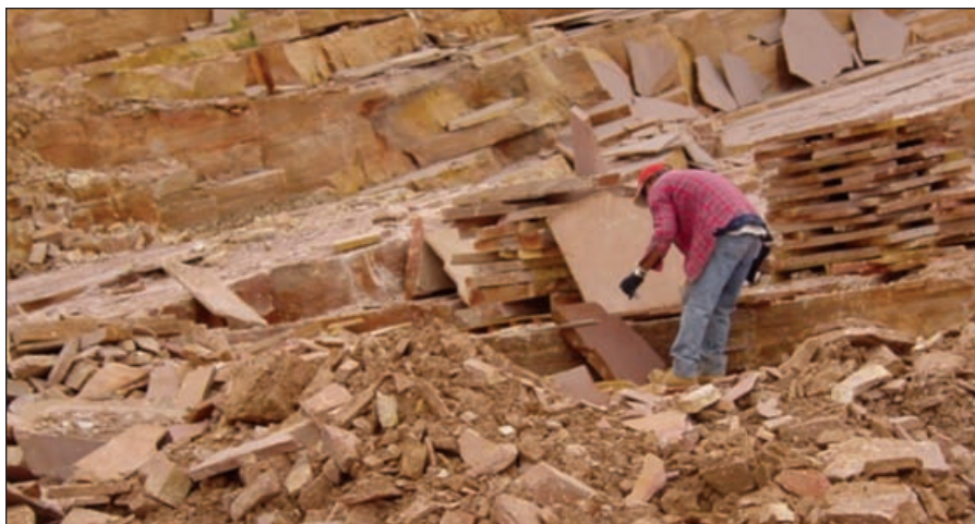
Figure 78. Worker shapes flagstone from the Lyons Sandstone in the quarry near Lyons in Boulder County. The stone is used as flagstone for buildings, walls, walkways and other decorative purposes.
