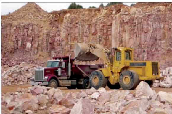
Figure 74. Operations at the Table Mountain Quarry, Fremont County, owned by Continental Materials, Inc. This quarry produces rock from the Dakota Sandstone, an extremely hard, durable material, good for use as rip-rap and road base.
