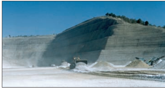
Figure 82. A dozer operates at the highwall of American Gypsum’s Eagle County mine. The gypsum from the mine supplies raw material for the drywall plant adjacent to the mine, fabricating gypsum wallboard for construction in the Colorado region.
