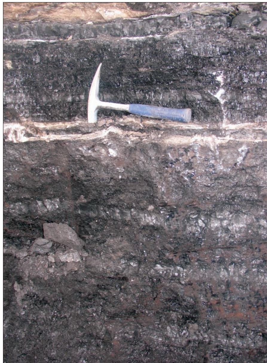
Figure 41. Detailed view of the lower Dakota coal bed at the New Horizon Mine surface high-wall. Note tonstein or ash beds interbedded within the coal unit near hammer. These ash beds are usually cleaned out during coal washing in preparation plants or at the power plant environmental controls.
