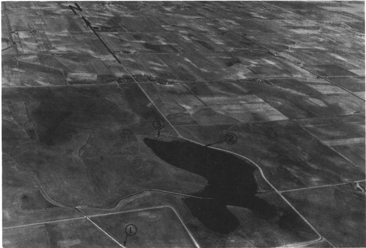
FIGURE 12.— Aerial view of the Olds Reservoir area illustrating the location of the inflow station 1 , the Olds Reservoir staff gage 2 , and the observation well B1-63-21daa 3 .
