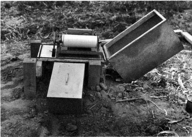
Figure 6. Continuous water level recorder installed on an observation well.
