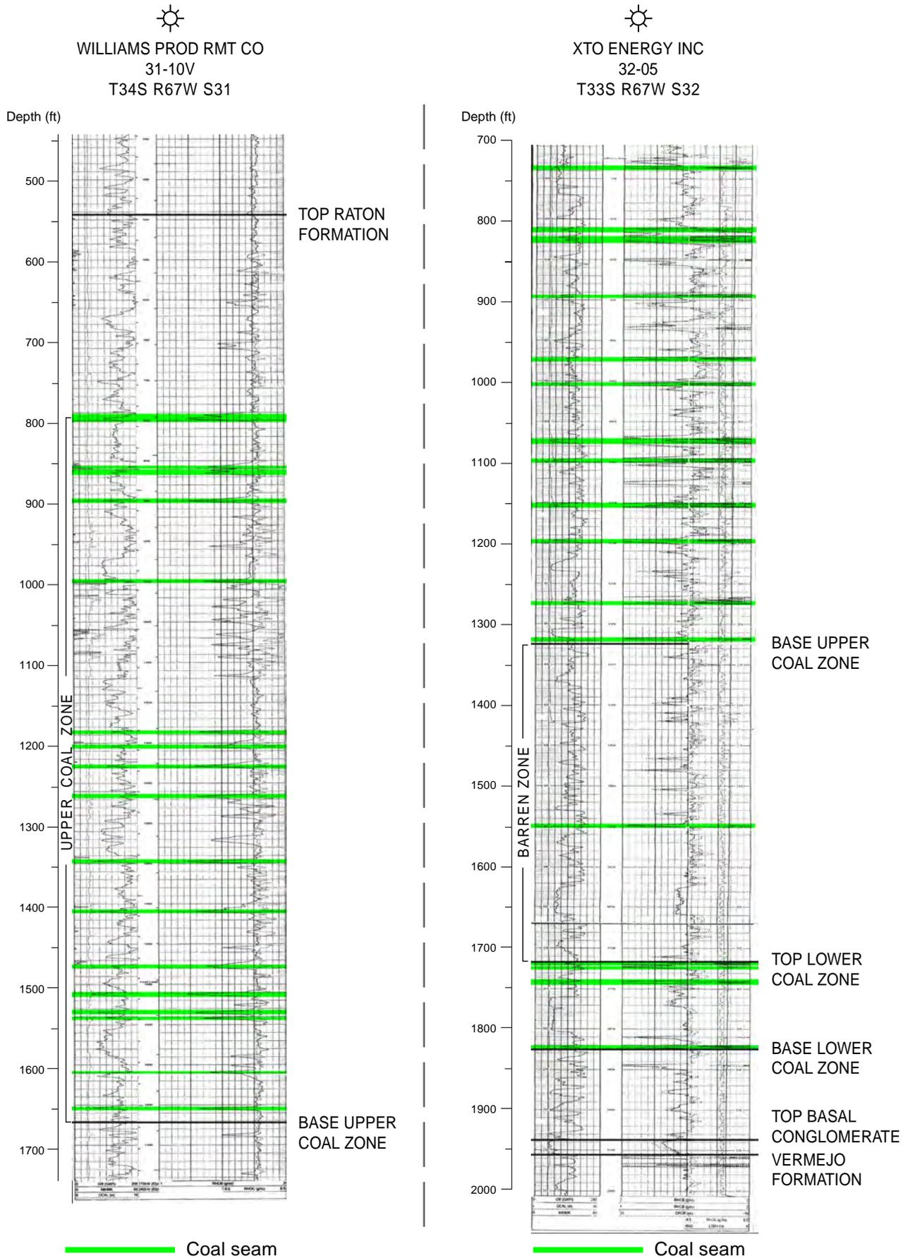
Figure 4.3 Type Geophysical Log for the Raton Formation Coal Zones from Separate Wells
