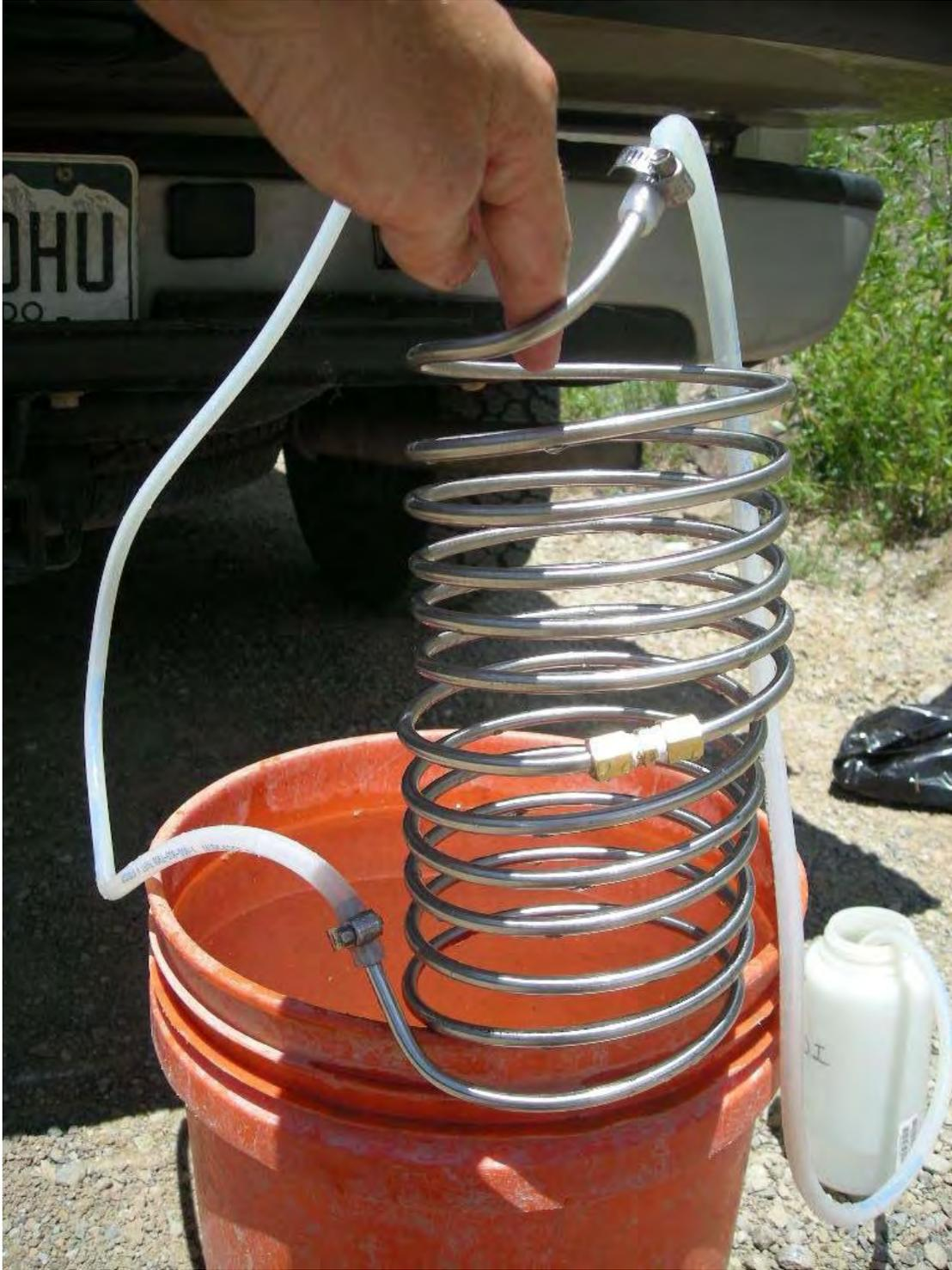
**Figure 5.** Stainless steel cooling coil, which is immersed in a bucket filled with ice and water during sampling. The brass fitting visible in the photo is a union fitting that allows two pieces of tubing to be joined together to form a longer (~16 ft), continuous coil.
