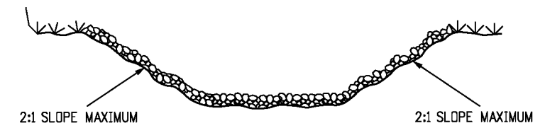
SECTION C-C RIPRAP-LINED DITCH
