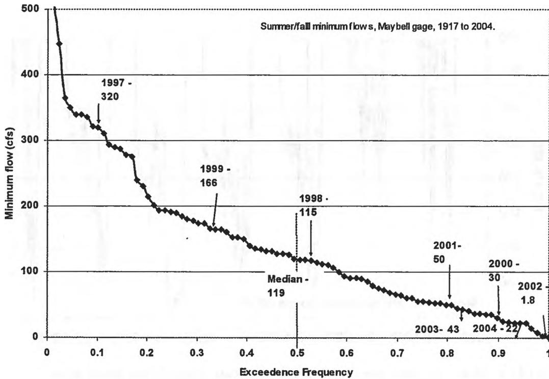
Figure A2-2. Exceedence probability values for summer/fall minimum flows, Maybell Gage, Yampa River for the period of record (1917-2004).
