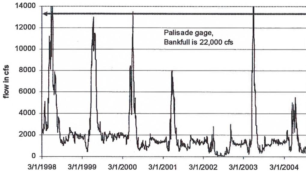
Figure A2-7. Annual hydrograph from 1998 to 2004, Palisade Gage, Colorado River.
