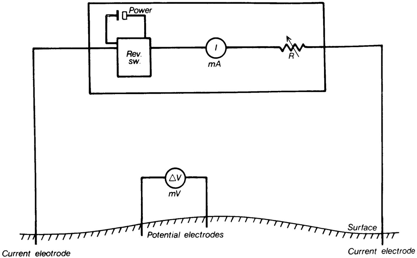
Figure 28. Schematic diagram for resistivity (from J. Combs, 1980).
