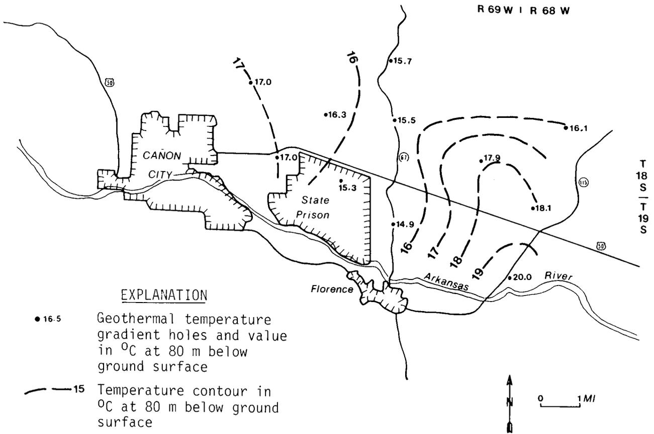
Figure 4. Temperatures at a depth of 80 meters.
