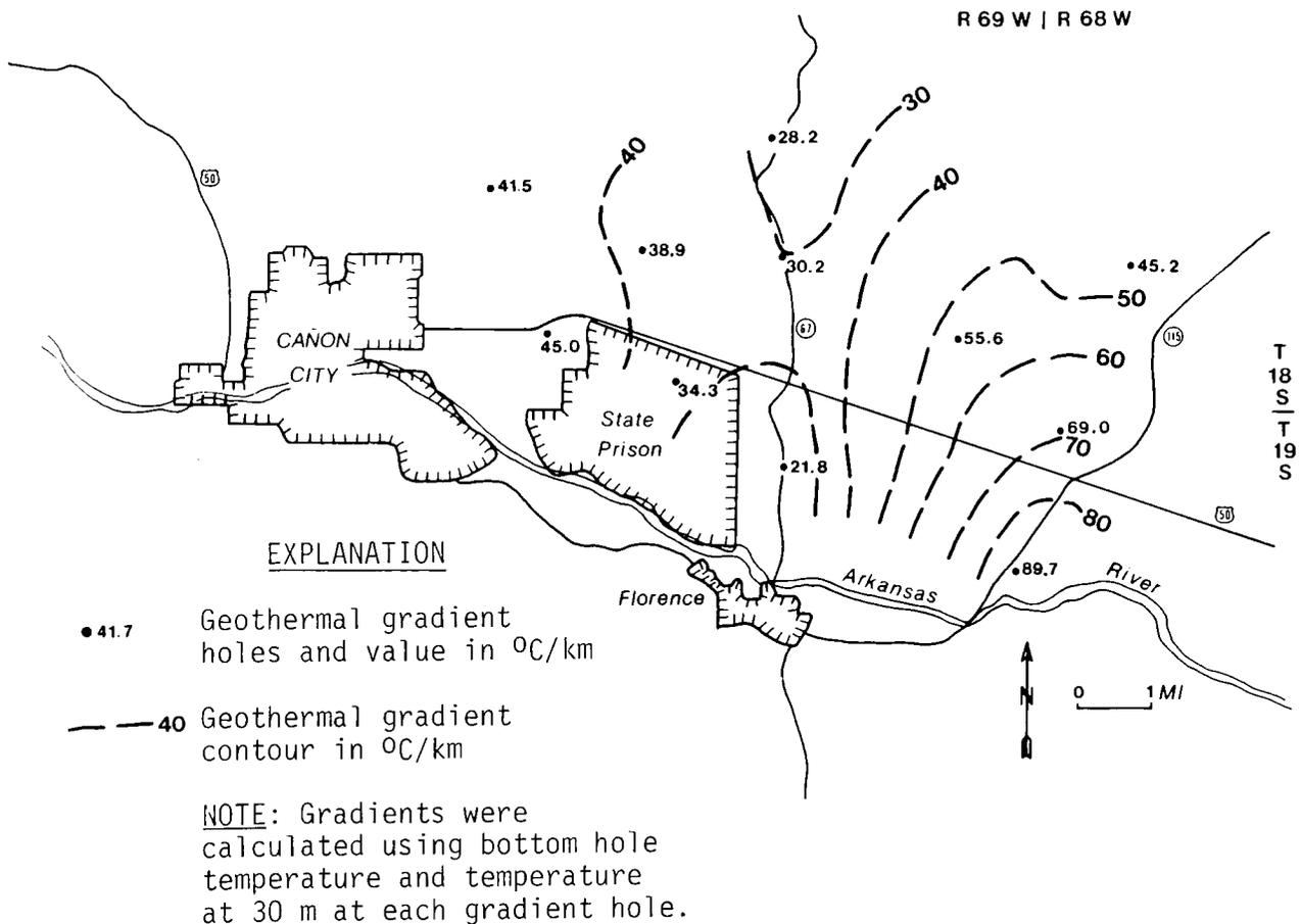
Figure 3. Geothermal gradient holes and measured values.
