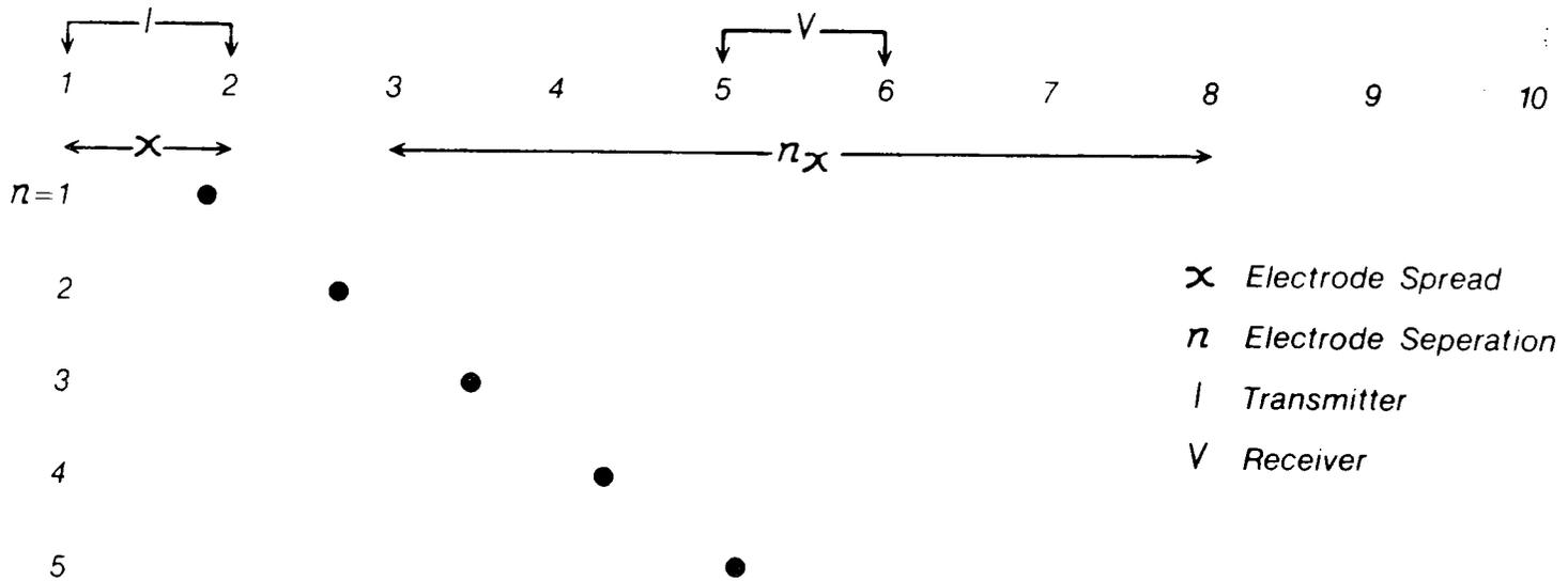
Figure 33. Typical dipole-dipole array (from J. Combs, 1980).
