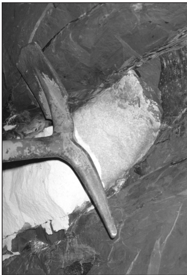
Figure 20. Photograph showing a convex upward pressure point (slickensided) along the roof rock of the Roadside Mine that formed from the light colored dike material. Observe the dark-gray, millimeter-scale, claystone clasts in the dike material adjacent to the roof rock.
