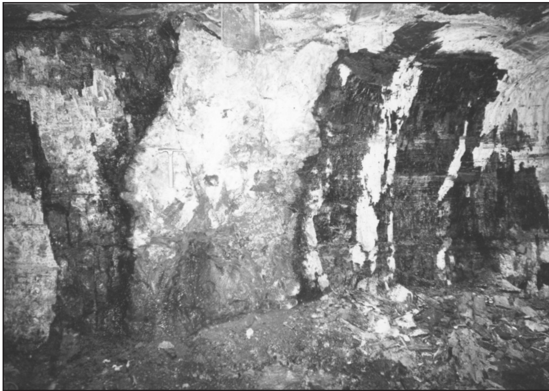
Figure 21. Photograph showing a columnar-shaped dike, more than a meter thick, in the Cameo No. 1 Mine. The rock hammer on the left side of dike is about 25 cm long.
