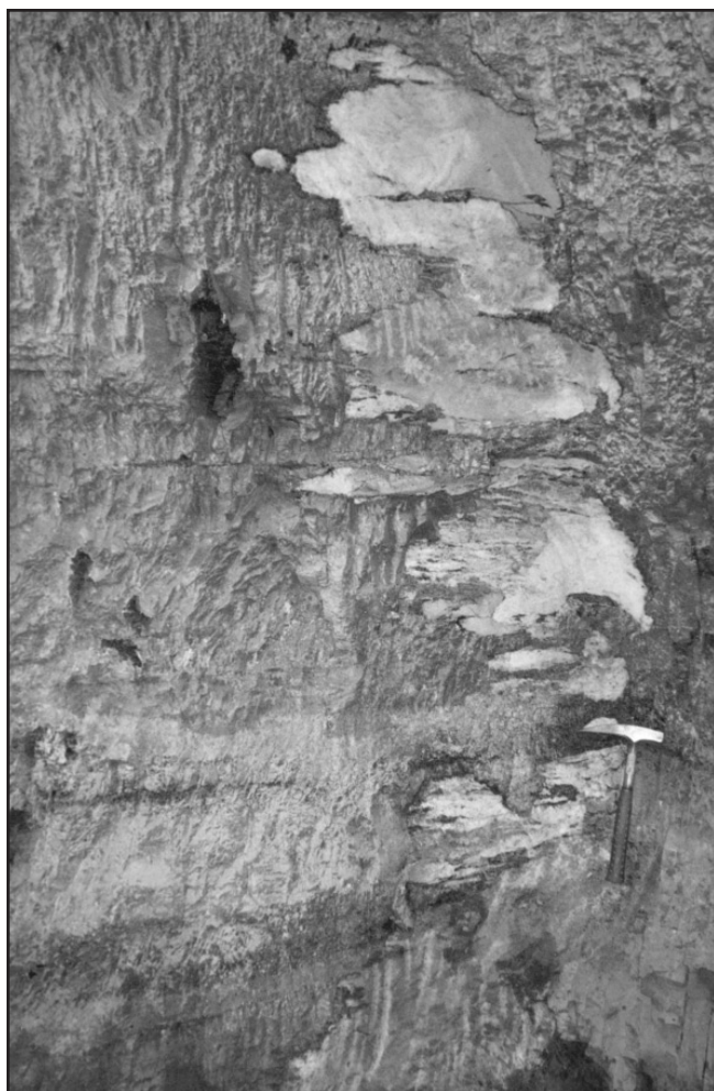
Figure 17. Photograph showing the smooth contacts and the discontinuous, crenulated character of a sigmoidal-shaped dike in the West Elk Mine.
