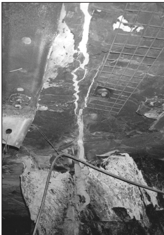
Figure 14. Photograph of dike material that formed a zig-zag pattern across the roof of the Cameo No. 1 Mine and that resemble infilled fractures.
