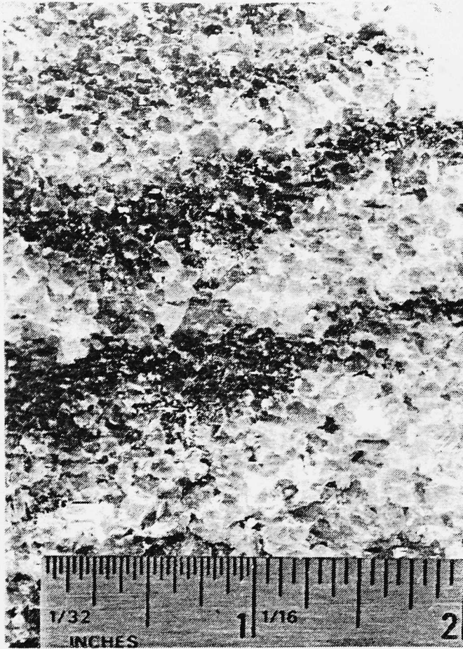
Figure 8: Close-up of banded marble. Note variable grain size and alternating coloration. Brown staining is due to the weathering of fine pyrite located between grains. Banded marble beds are generally too thin and too folded to be of economic importance.
