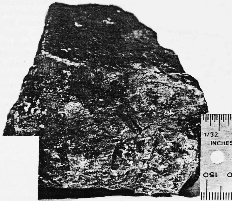
Figure 5. Hornfels from the Conundrum-Colorado Highland property. This metamorphic rock is interbedded with marble and was produced from a carbonaceous sandy shale parent rock. Hornfels at the Colorado-Highland property is of no economic importance. Note iron staining caused by fine pyrite inclusions in the rock. Number corresponds to sample number in Appendix A.
