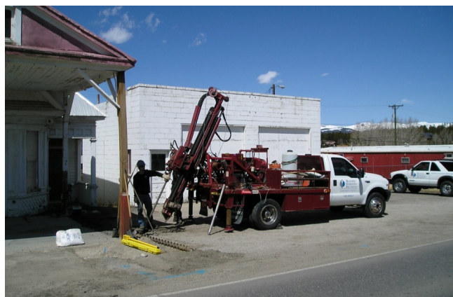
Soil probing is an effective way to gather soil and groundwater samples.
