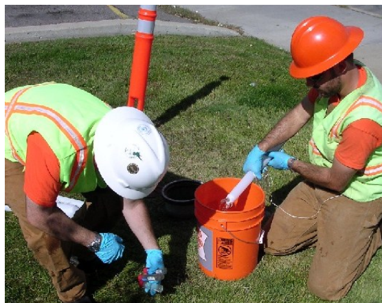
Groundwater sampling using disposable bailers.
