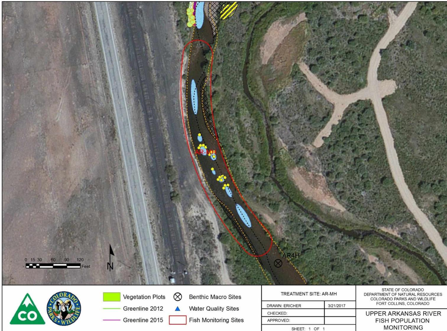
Figure C.5. Aerial image showing habitat treatments within fish monitoring site AR-MH on the Upper Arkansas River.
